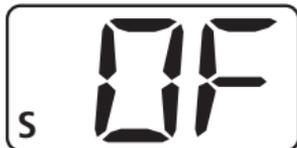
3. Press the ▲ or ▼ keys to select the required CTCSS tone. The flashing 'S' indicates the tones you are selecting are CTCSS tones.
