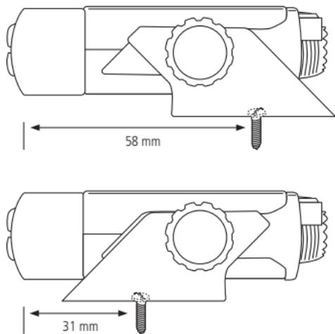
The mounting bracket can be oriented with the arms extending either forward or backwards to adjust the position of the front panel with reference to the mounting point.
